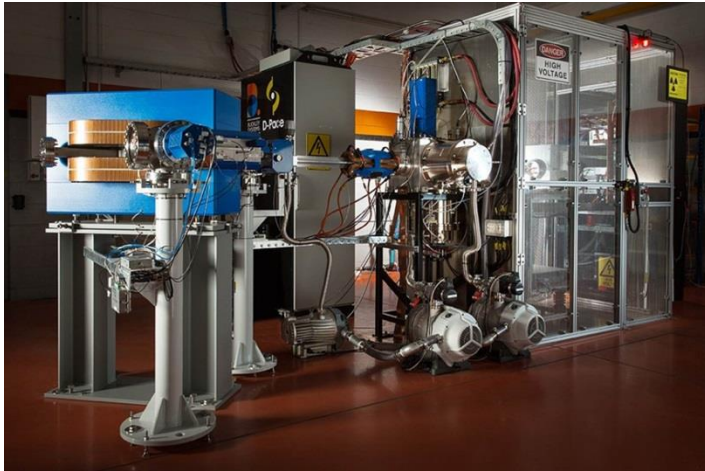
Turnkey Ion Source Including Optional Beamline and Mass Spectrometer
