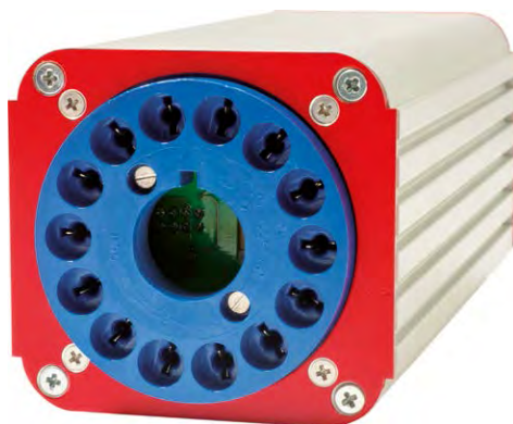
gamma stream rear view. Internal divider can be adapted for NaI(Tl), LaBr 3 (Ce), CeBr 3 detectors with standard 14-pin and 10-8 stages PMTs.
