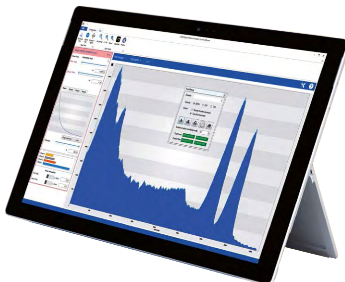
Screenshot of an emulated spectra in the graphical user interface provided with the Digital Detector Emulators.
